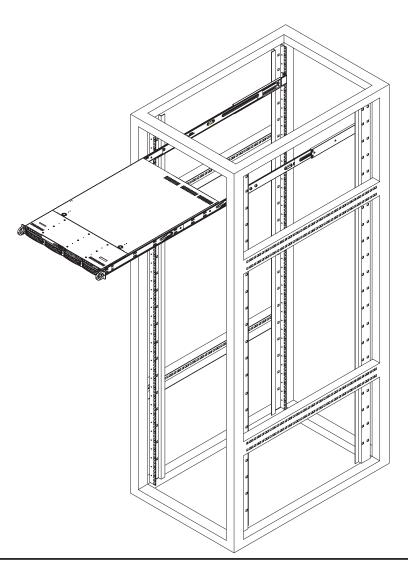
Figure 2-3. Installing the Server into a Rack
